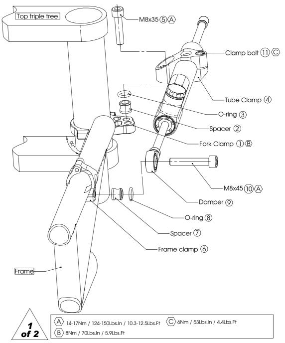
See WWW.HYPERPRO.COM for the latest pictures, modifications, specs. and e-drawings of this steering damper kit.
